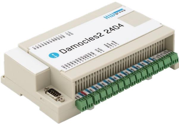
Secure industrial I/O device with PoE and Telco -48 V power options.
