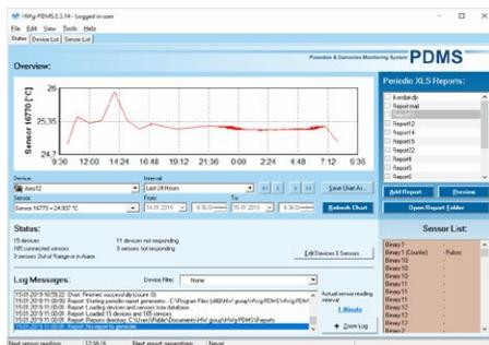
*Windows application for collecting data from sensors and inputs over LAN and GSM. Export of data in the background.*
