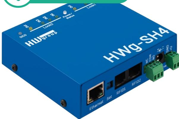
Main control unit for access control systems, compatible with any RS-232/Wiegand RFID reader and lock.
