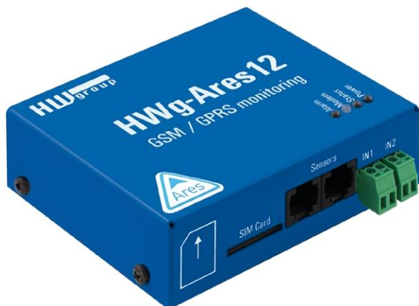
*Industrial measuring and monitoring device for 14 sensors with GSM communication and back-up power.*
