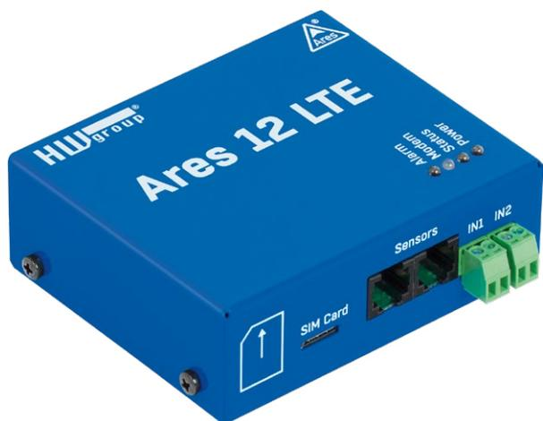
*Industrial measuring and monitoring for 14 sensors with GSM and LTE communication and back-up power.*
